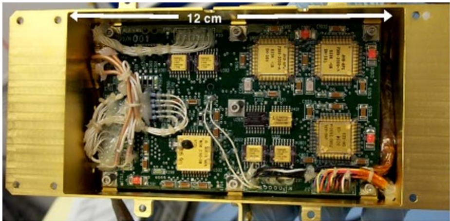
Fig. 10 MLA Range Measurement Unit (RMU) assembly shown mounted in its beryllium housing
