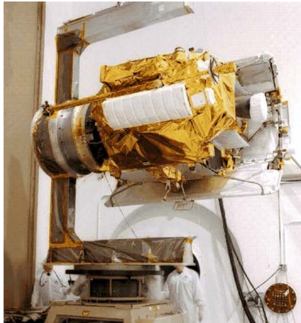
Fig. 7 MESSENGER in post-launch configuration during mass properties testing
