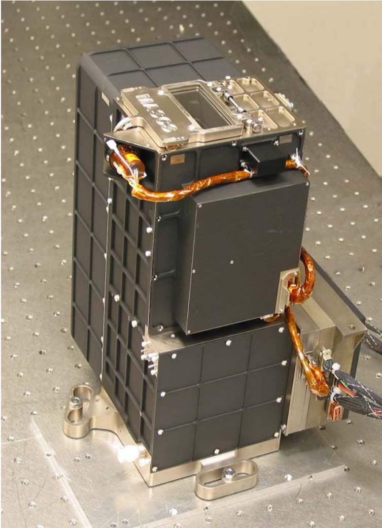
Fig. 1 MASCS instrument image taken during instrument testing at the Laboratory for Atmospheric and Space Physics (LASP) at the University of Colorado
