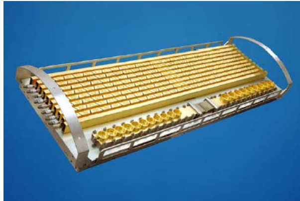
Fig. 4 A MESSENGER phased-array antenna and fanbeam antenna. Eight slotted waveguide antennas comprise the phased-array antenna. The fanbeam antenna is comprised of two helix arrays (uplink and downlink). The overall dimensions of the assembly are 28 cm by 81 cm
